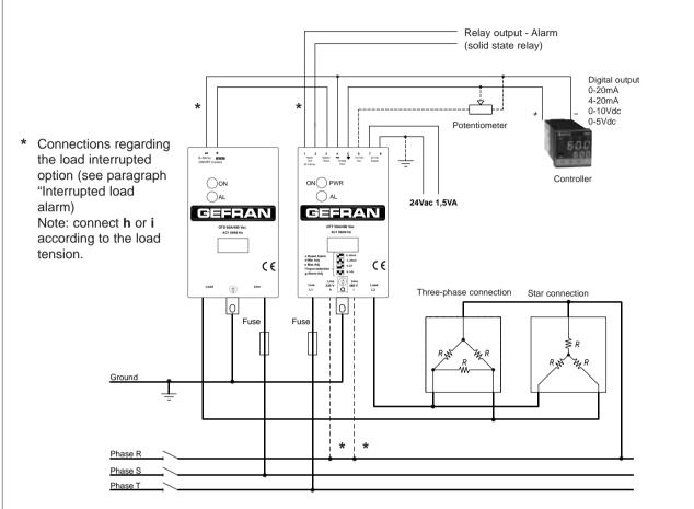
Three-phase star connection with neutral using one GTT in Master configuration and two GTSs in Slave configuration.
